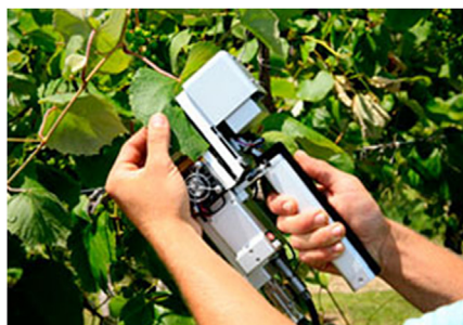
Fig. 6. An example of photosynthesis measurement system and an illustration of A-C_i curve based on FvCB model. A-C_i curve is one of key response curves to be measured in the field.
